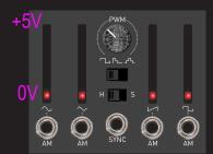
Four channel mixer with linear control VCA's sums sine, triangle, saw, pulse waveforms expecting external unipolar signals to mute them eventually with high events.
